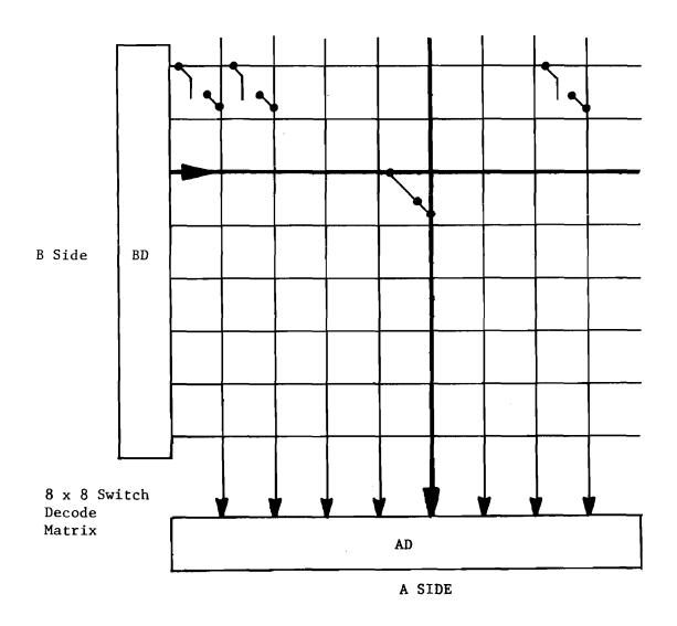
Keyboard Encoding Matrix Diagram
