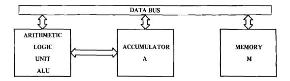
Partial Block Diagram including Arithmetic Logic Unit of MCS650X FIGURE 2.2
